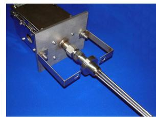
A total of six 3.0mm diameter type 'K' thermocouples were held within 6.0mm diameter support tubes with each tube and thermocouple terminating at predetermined lengths. The support tubes were angled at their exit to enable the thermocouples to be pushed out the tube exit and against the inner wall of the dip pipe, prior to being held firmly by a sealing gland beneath the terminations enclosure.
